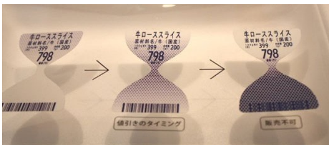
Figure 7: An hour glass shaped sensor for determining the spoiling of meat, as the meats get rotten the sensor changes colour from white to black completely covering the bar code so it cannot be scanned.
